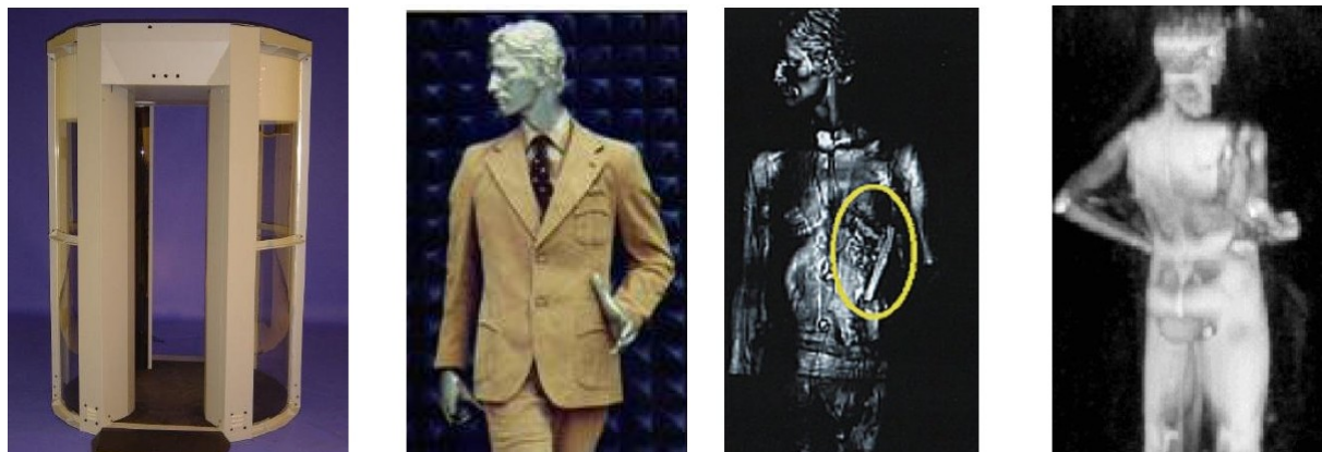
Fig. 1. Millimeter-wave imaging technology. From left to right: security entry portal SafeScout100 of SafeView; example of a clothed dummy and its millimeter-wave image showing a gun concealed under the clothing; image representation of 3D volumetric data of a real person.
