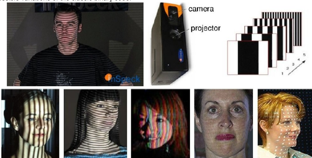
Fig. 1. Top: White light projection method. Left: projection of light pattern as stripes. Center: scanning device Capturor of InSpeck. Right: projected sequence of binary coded stripes pattern. Bottom: Examples of projected light pattern. From left to right: vertical stripes by 3D-Shape, horizontal lines by Wicks and Wilson, color coding by Sanyo Electric, squared pattern by Eyetronics, dot pattern by VX Technologies.
