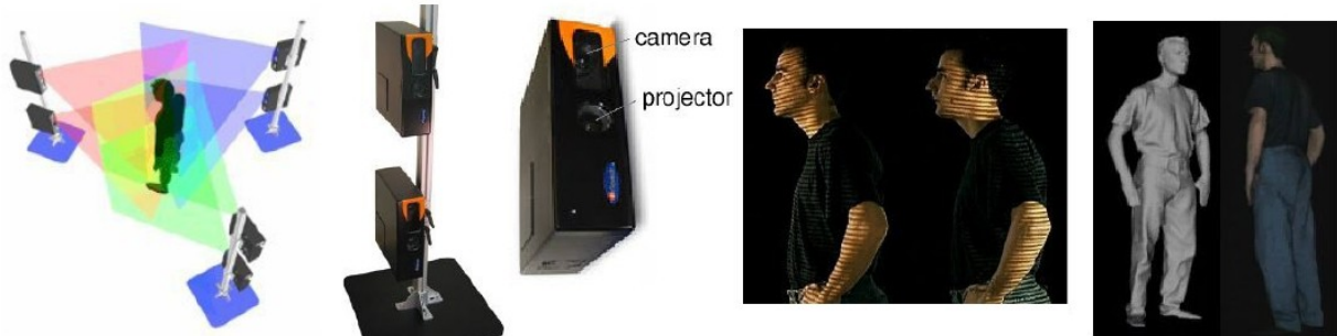
Fig. 2. Full body scanner of InSpeck. From left to right: configuration with six units; column with two acquisition units; unit composed of one camera and one projector; coded light projection, resulted 3D surface model.
