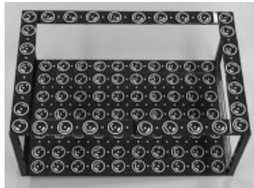
Fig. 6: 3-D calibration frame with coded targets
