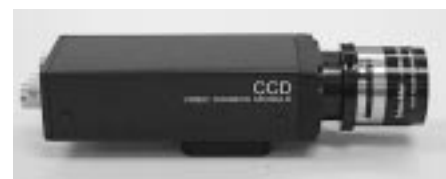
Fig. 2: CCD camera with 35 mm lens
