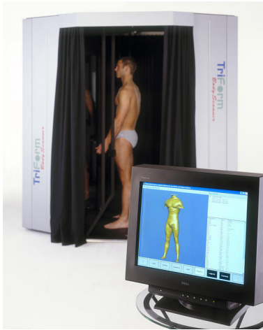
Figure 7. Scanning systems with projection of light patterns: full body scanner TriForm of Wicks and Wilson.
