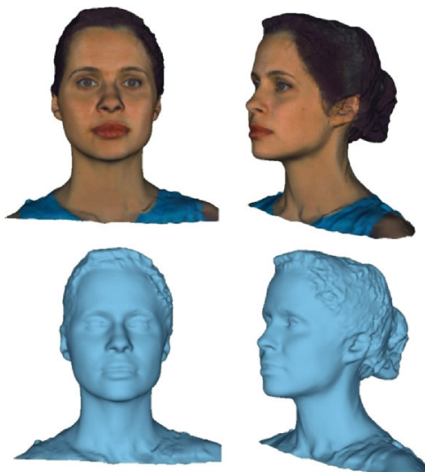
Figure 12. Examples of 3D scanning data: head model (with and without texture) resulted by using InSpeck head scanner system.
