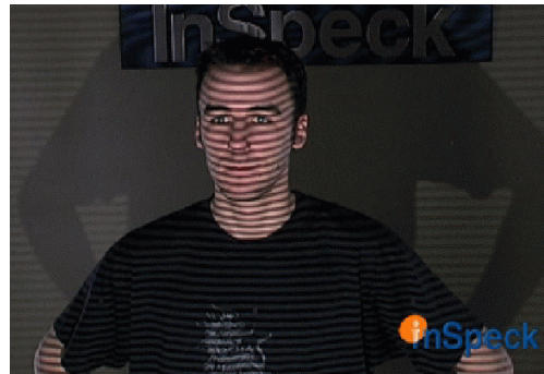
Figure 4. Projection of light pattern as stripes (image of InSpeck).
