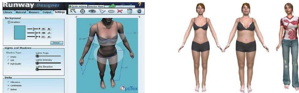
Fig. 21. Left: parametrized virtual human body model used in virtual-try-on application, Runway 3D of OptiTex Ltd. (Israel). Right: virtual anthropometric mannequins based on anthropometric data, from IFTH (France).
