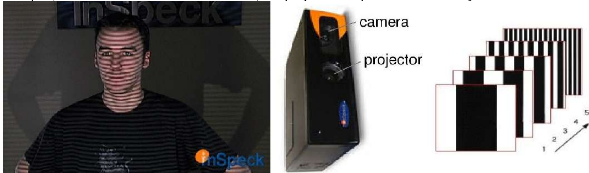
Fig. 6. Left: projection of light pattern as stripes. Center: scanning device Capturor of InSpeck Inc. (Canada). Right: projected sequence of binary coded stripes pattern.
