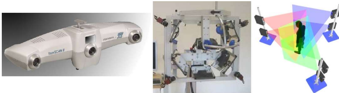
Fig. 8. White light projection systems. Left: face scanner faceSCAN-II of Breuckmann GmbH (Germany), with two cameras and one projector. Center: face scanner Gscan of IVB GmbH (Germany), with one projector, five cameras and mirrors system. Right: full body scanner Mega 3P of InSpeck Inc. (Canada) with six units, each with a camera and a projector.
