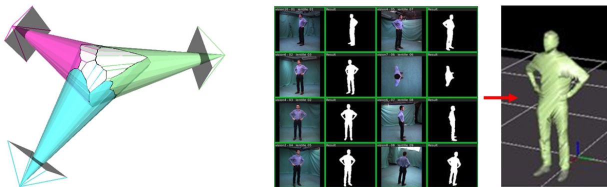
Figure 8: Left: principle of the visual hull method. Right: example of 4D capture system based on visual hull, 4DV Classic of 4D View Solutions [11].
