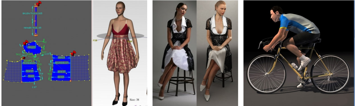
Figure 16: Virtual-try-on by 3D Runway of OptiTex Ltd. (Israel). From left to right: 2D patterns; 3D visualization of the final garment; comparison real-virtual; dynamic simulation.
