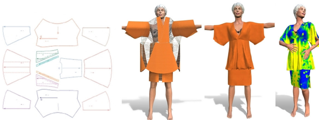
Figure 15: Example of virtual-try-on solution Vidya of Assyst-Bullmer [18]. From left to right: 2D patterns of the different cloth parts; parts placed and stitched around the body model; final result of the cloth simulation; analysis of the tensions in the cloth.
